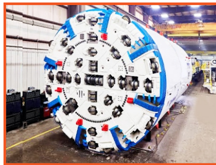
Tunnel Boring Machine (TBM)
